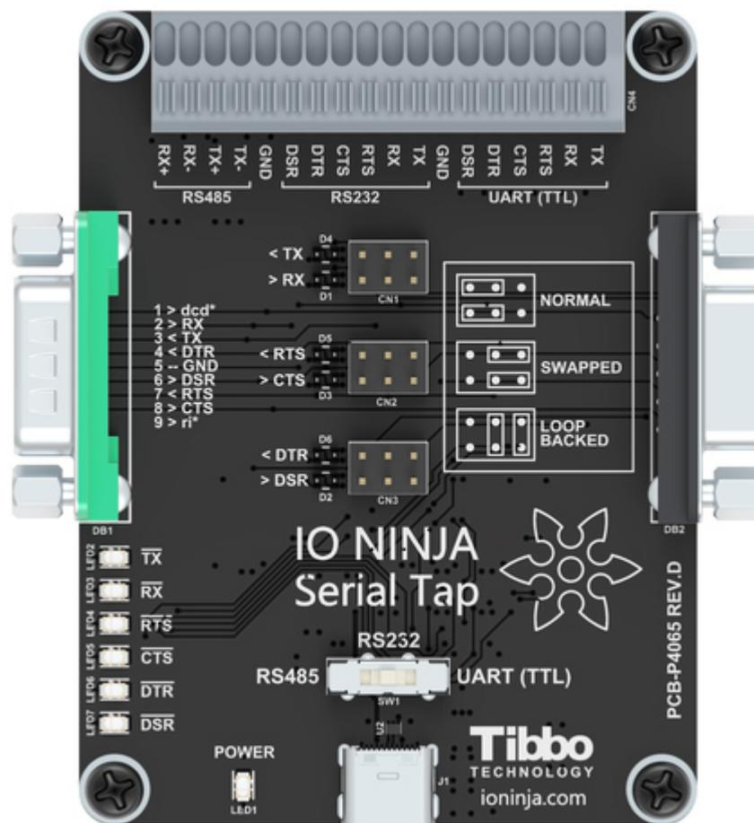
Serial Tap is an affordable serial sniffer that can monitor RS232, RS485, and TTL-level UART communications. The Tap connects to your PC via a USB cable and is compatible with IO Ninja terminal/sniffer software.
