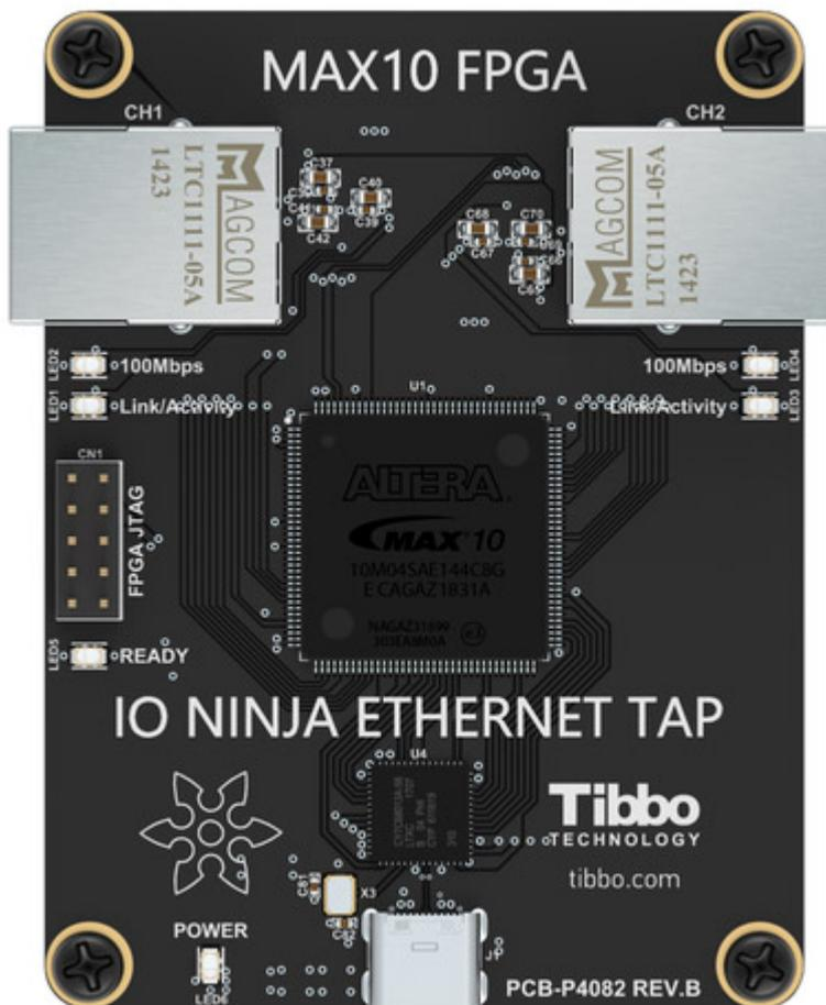
Ethernet Tap is an affordable sniffer for monitoring Ethernet traffic flowing through a single Ethernet connection. To monitor Ethernet traffic, an Ethernet cable that was initially connecting a switch (hub) to an Ethernet device is replaced by two Ethernet cables and the Ethernet Tap is inserted between them, in what is known as a
